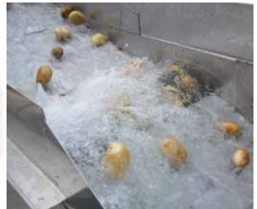
Stones and mud clods sink down the stone chute whereas produce floats over the space and continues down the processing line
