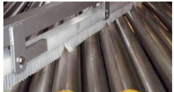
Cleaning system for round stainless steel rollers
