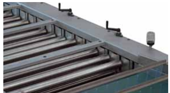
Manual handles for size adjustment and oil reservoir for chain lubrication
